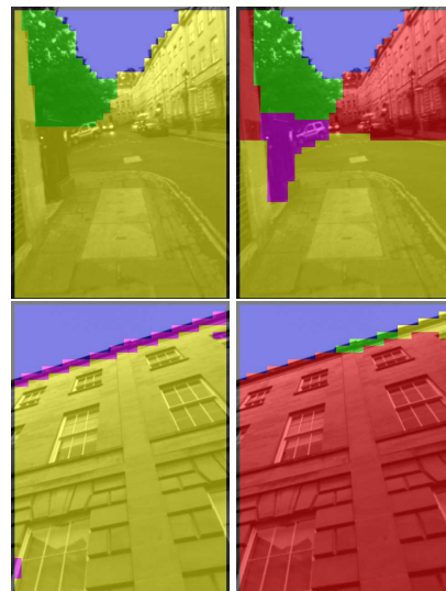
Figure 1: Typical results of our algorithm, showing how segmentation results using only vision (left) can be improved by taking into account the camera orientation (right). In both examples knowledge of the camera orientation avoids misclassifying vertical walls as ground (yellow). See Fig. 7 for full colour legend. All images are best viewed in colour.
